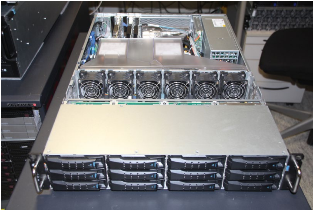
Picture 2: SB202-TU head node server from AIC
