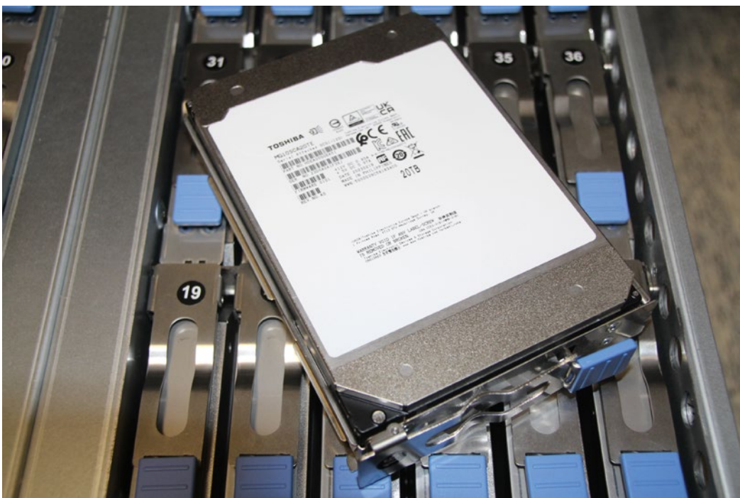
Picture 5: Toshiba MG10SCA20TE HDD in Promise tray
